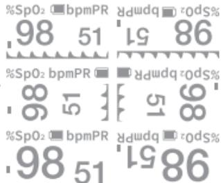
Press the power button continuously during the monitoring process. The data monitored and display method will be displayed cyclically on the OLED screen in two different ways (text & graph) and in four directions, as shown in the illustration below.
