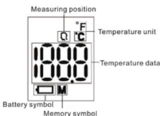
Location indication: The icon indication the correct measuring position when measuring.
